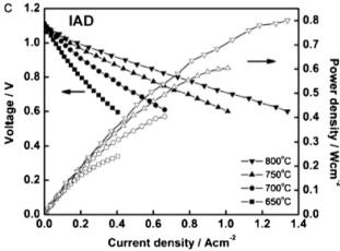
Fig. 34 I-V curves of cells fabricated from GDC deposited by (a) screen printing (b) electron beam evaporation (c) ion assisted deposition. Reproduced with permission from ref. 85 Copyright 2011 Elsevier.
