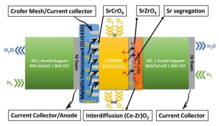
Fig. 2 Illustration of degradation issues and their source in a typical SOFC stack.
