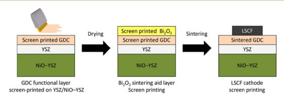
Fig. 29 Fabrication route of deposition of sintering aid ( $Bi_2O_3$ ) on GDC interlayer. (Reproduced with permission from ref. 30 Copyright 2022 Elsevier.)
