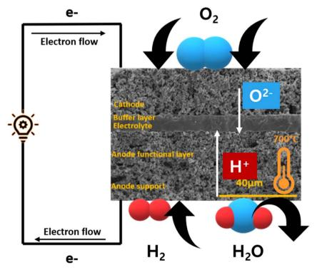
Fig. 5 Schematics of a typical O<sup>2-</sup> conducting SOFC.
