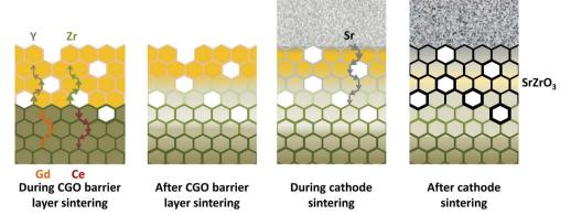
Fig. 12 Illustration of the migratory pathways from the GDC interlayer sintering to the cathode and formation of secondary phase. (Reproduced with permission from ref. 51 Copyright 2021 Elsevier.)
