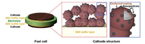
Fig. 19 Schematics of an LSCF electrode backbone with nanoparticles. (Reproduced with permission from ref. 114 Copyright 2017 Royal Society of Chemistry.)
