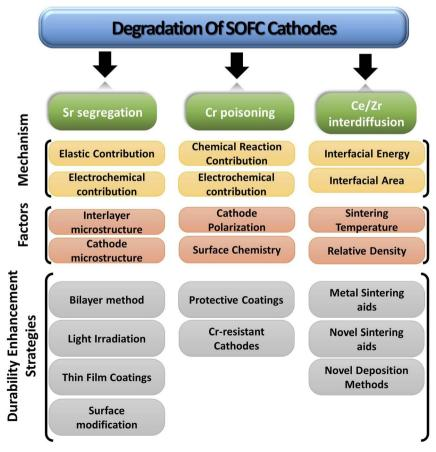
Fig. 4 Simplified overview of degradation of SOFC cathodes.
