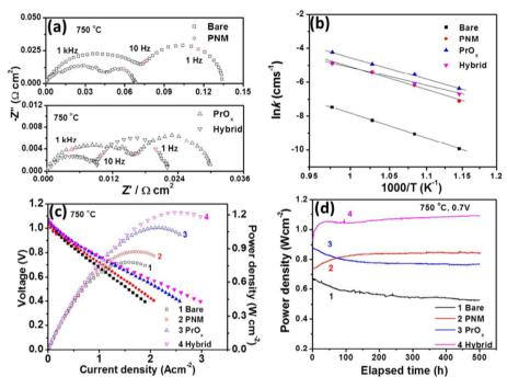
Fig. 20 (a) Impedance spectroscopy of bare cathode and PMN cathode (b) conductivity plot (c) *I–V* curves (d) peak power density over time. (Reproduced with permission from ref. 114 Copyright 2017 Royal Society of Chemistry.)
