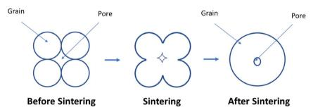
Fig. 10 How pore size reduces during sintering process.
