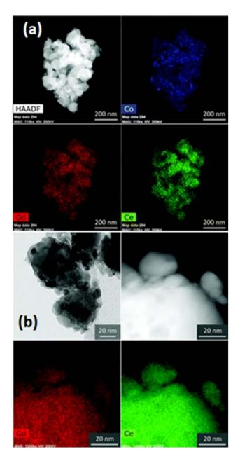
Fig. 14 TEM imaging of the morphology and nanoparticle distribution of bilayer from (a) top and (b) bottom. (Reproduced with permission from ref. 32 Copyright 2018 Royal Society of Chemistry.)
