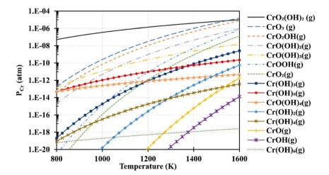
Fig. 6 Using Ebbinghaus's thermodynamic data,  $^{93}$  partial pressures of several gaseous chromium species over a  $Cr_2O_3(s)$  source were computed for 1 atm humidified air. (Reproduced with permission from ref. 92 Copyright 2020 Elsevier.)
