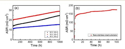
Fig. 24 (a) In situ monitored ASR values for spinel coated samples at 700 °C for up to 1000 h and (b) ASR of the uncoated 460FC stainless steel substrate, measured under a current load of 10 mA cm<sup>-2</sup>. (Reproduced with permission from ref. 122 Copyright 2022 Elsevier.)
