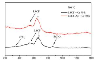
Fig. 26 Typical Raman spectra of LSCF and LSCF-Ag cathodes after the Cr treatment at 700 °C for 40 h. (Reproduced with permission from ref. 123 Copyright 2022 Elsevier.)
