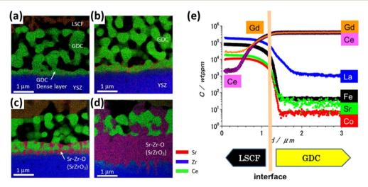
Fig. 11 (a)—(d) STEM-EDS of LSCF/GDC/YSZ at 0.5 h, 1 h, 2 h, 16 h to reflect the interdiffusion of Zr, Ce and Sr. (Reproduced with permission from ref. 109 Copyright 2017 Elsevier.) (e) SIMS depth profile of LSCF/GDC diffusion couple to evaluate interdiffusion. (Reproduced with permission from ref. 87 Copyright 2011 Elsevier.)
