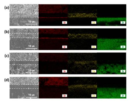
Fig. 31 EDS mapping of cross-section side of GDC: (a) sintered at 1000 °C and (b) 1200 °C; GDC with  $Bi_2O_3$  layer (c) sintered at 1000 °C and (d) 1200 °C. (Reproduced with permission from ref. 30 Copyright 2022 Elsevier.)
