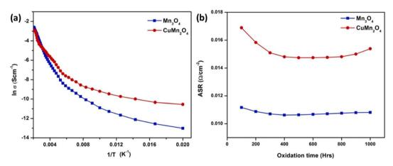
Fig. 23 (a) Arrhenius plot shows  $CuMn_2O_4$  has higher electrical conductivity (b) ASR measurement of  $Mn_3O_4$  and  $CuMn_2O_4$  coated SUS430. (Reproduced with permission from ref. 117 Copyright 2022 Elsevier.)
