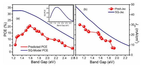
Fig. 7 Illustration of results of XGBoost model used in this work for predicting band gap and PCE and their comparison with theory. Panel (a) and (b) exhibits the comparisons of the predicted PCE and current density respectively with the limit proposed by Shockley and Queisser in their theory, brown and yellow lines represent the maximum PCE. The insets show the reduced size curves of the S–Q theoretical limit.
