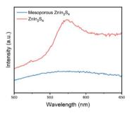
Fig. 5 Stead-state PL spectra of mesoporous Znln<sub>2</sub>S<sub>4</sub> and Znln<sub>2</sub>S<sub>4</sub>.
