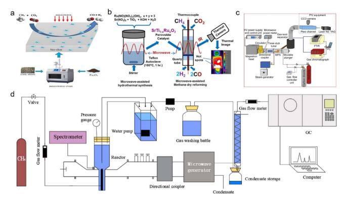
Fig. 3 (a) Porous Fe-rich biomass-derived carbon<sup>142</sup> and (b) ruthenium-doped strontium titanate (SrTiO<sub>3</sub>) perovskite<sup>143</sup> catalysts applied for microwave-assisted methane dry reforming. (c) and (d) Sketch of microwave plasma enhanced hydrogen production *via* the steam reforming of methane.<sup>144,145</sup>
