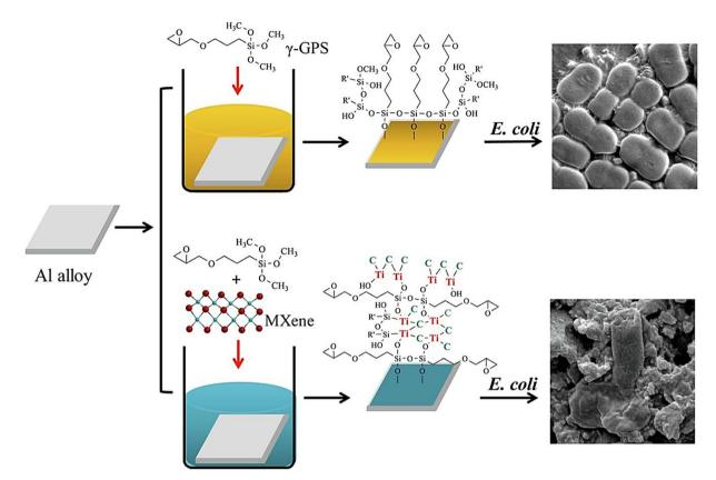
Fig. 6 MXene-hybridized silane films with antibacterial properties; MXene ( $Ti_3C_2$ ) sheets were hybridized into the  $\gamma$ -glycidoxypropyltrimethoxysilane (y-GPS) film on AA2024 aluminum (Al) alloy surface. Reproduced with permission from ref. 27 Copyright 2020 Elsevier.
