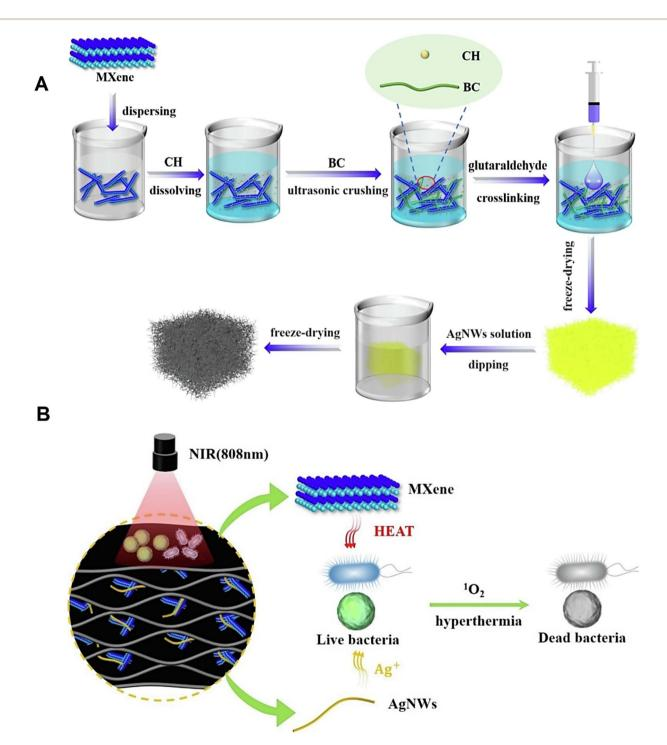
Fig. 5 (A) The preparative process of composite aerogel from bacterial cellulose (BC), chitosan (CH), MXene, and silver nanowires (AgNWs). (B) The antibacterial mechanisms of the composite aerogel against pathogenic bacteria. Reproduced with permission from ref. 81 Copyright 2022 Elsevier.
