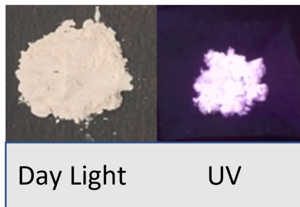
Fig. 1 Image of \text{Na}_3\text{Ba}_2\text{LaNb}_{10}\text{O}_{30}\text{:xDy}^{3+} ( x = 7 mol%) phosphor sample under daylight and 365 nm UV light.
