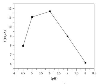
Fig. 11 pH effect of parathion (3.43  $\times$  10<sup>-5</sup> M) on peak current at fabricated poly(safranine) film under scan rate: 100 mV s<sup>-1</sup>. This figure has been adapted/reproduced from ref. 35 with permission from Hindawi, copyright (2023).
