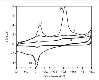
Fig. 10 Voltammogram response of parathion (1.9  $\times$  10<sup>-5</sup> M) at (a) bare electrode (GCE), (b) poly(safranine) film-modified electrode. This figure has been adapted/reproduced from ref. 35 with permission from Hindawi, copyright (2023).
