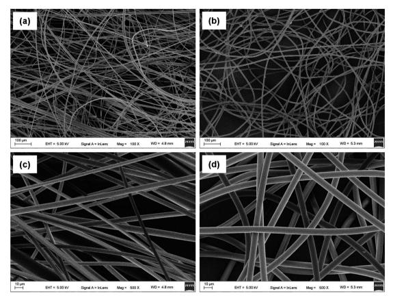
Fig. 2 SEM images of the PS-Eu<sub>1</sub>-Tb<sub>60</sub> fiber membrane (a and c) and the neat PS fiber membrane (b and d).
