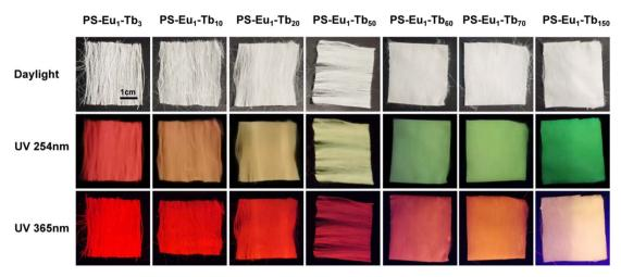
Fig. 5 Digital images of the UV-excited dual-mode luminescent electrospun fiber membranes under daylight, 254 nm light and 365 nm light, respectively.
