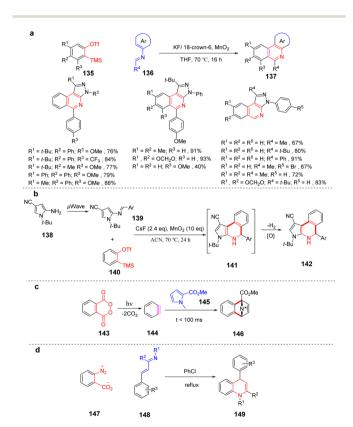
Scheme 21 DA reaction of benzyne with nitrogen-containing dienes. (a) Synthesis of isoquinolines *via* the oxidative aza-DA reaction, (b) synthesis of pyrrolo[2,3-c]isoquinolines scaffold *via* aza-DA reactions, (c) photolysis of a benzyne precursor, (d) synthesis of aryl-substituted 1,4-dihydroquinolines by [4 + 2] cycloaddition.
