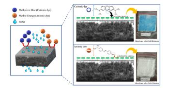
Fig. 10 Dye removal scheme.
