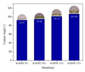
Fig. 5 Contact angles of the membranes.
