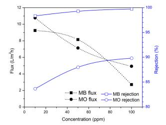
Fig. 9 Performance of the R-HDPE 15% membrane for MO and MB removal.
