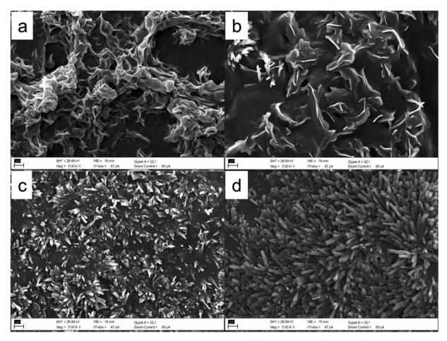
Fig. 2 SEM micrographs of wheat straw wax recrystallized by different solvents, (a) petroleum ether, (b) toluene, (c) TMO, and (d) DEDMO. Scale bars: 1 µm.
