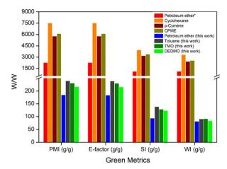
Fig. 1 Green metrics (PMI, E-factor, SI, and WI) for literature process and the processes developed in this work. \* based on Asemave et al.<sup>29</sup>
