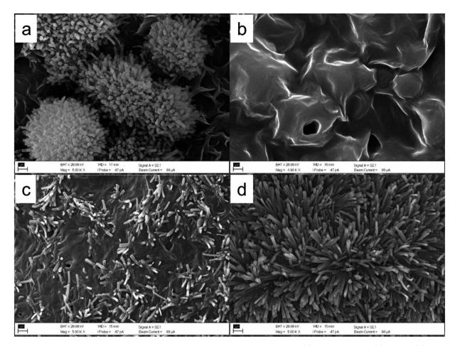
Fig. 3 SEM micrographs of hentriacontane-14,16-dione recrystallized by different solvents, (a) petroleum ether, (b) toluene, (c) TMO, and (d) DEDMO. Scale bars: 1 µm.
