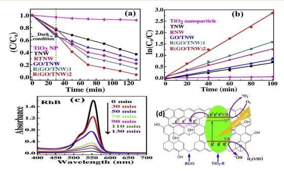
Fig. 9 (a) Plot of  $(C/C_0)$  versus time for degradation of RhB in the visible light, (b) kinetics of photodecomposition of the prepared samples, and (c) the absorption spectra of RhB under visible light irradiation catalyzed by R(GO/TNW)2 composite, and (d) schematic diagram elucidating the mechanism of photocatalytic activity of R(GO/TNW)<sub>2</sub> reprinted with permission from ref. 78. Copyright 2022 Elsevier.
