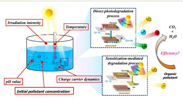
Fig. 10 Schematic shown of operational parameters affecting the photocatalytic degradation of organic pollutants.81
