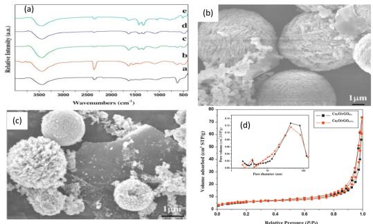
Fig. 2 (a) FT-IR spectra of as-prepared  $Cu_2O/rGO_{x\%}$  samples with various wt% of rGO, (b and c) FESEM image of  $Cu_2O/rGO$  0.05, and 0.5% (wt%), respectively, and (d)  $N_2$ -adsorption isotherms of  $Cu_2O/rGO_{0\%}$  and  $Cu_2O/rGO_{0.5\%}$  (wt) reprinted with permission from ref. 54. Copyright 2022 FISevier
