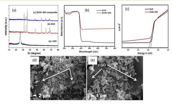
Fig. 4 (a) XRD patterns, (b) UV absorption spectra, (c) Tauc plot, and (d, e) FESM of synthesized samples reprinted with permission from ref. 65. Copyright 2022 Elsevier.
