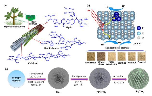
Fig. 1 (a) Chemical composition and structure of lignocellulose biomass. (b) Photocatalytic H<sub>2</sub> production from lignocellulose biomass over Pt nanocluster anchored porous TiO<sub>2</sub> microsphere photocatalysts. (c) Schematic illustration for the synthesis of Pt/TiO<sub>2</sub> photocatalysts.
