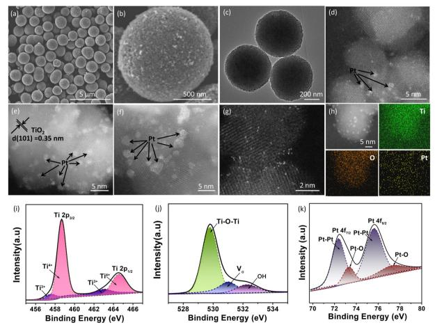
Fig. 2 (a and b) SEM and (c) TEM image of bare TiO<sub>2</sub>. (d-q) Spherical aberration-corrected HAADF-STEM image of 0.2% Pt/TiO<sub>2</sub> (d), 0.4% Pt/TiO<sub>2</sub> (e and g) and 1.0% Pt/TiO<sub>2</sub> (f). (h) HAADF-STEM and elemental mapping images of 0.4% Pt/TiO<sub>2</sub>. (i-k) High-resolution Ti 2p, O 1s and Pt 4f XPS spectra of 0.4% Pt/TiO<sub>2</sub>.
