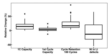
Fig. 7 Box-and-whisker plot of the relative change of 1C capacity (n = 16), first-cycle capacity (n = 22), capacity retention after 100 cycles (n = 22), and  $Ni_{ij}$  defects (n = 11) of Nb-doped LTMOs applied for LIBs.
