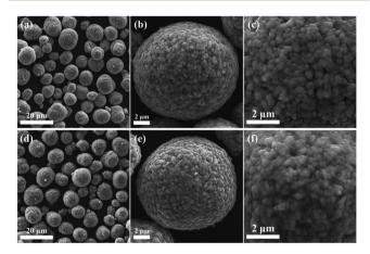
Fig. 1 (a–c) SEM images of a pristine  $LiNi_{0.6}Co_{0.2}Mn_{0.2}O_2$  (NCM622) sample. (d–f) SEM images of coated NCM622 prepared from a ball-milling method with  $Nb_2O_5$  (0.5 mol%). Reproduced with permission from ref. 76. Copyright 2021, Elsevier.
