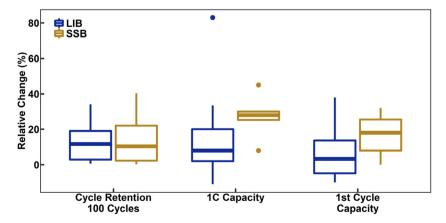
Fig. 5 Box-and-whisker plot of the relative change of capacity retention after 100 cycles, 1C capacity, and first-cycle capacity of LiNbO₃ coatings with respect to "bare" NCM CAMs for both LIB and SSB systems. For cycle retention, n = 19 and 9 for LIB and SSB, respectively. For 1C capacity, n = 17 and 6 for LIB and SSB, respectively. For first-cycle capacity, n = 18 and 11 for LIB and SSB, respectively.
