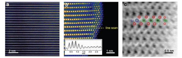
Fig. 8 STEM images of Nb-doped  $Li_{1.2}Mn_{0.54}Ni_{0.13}Co_{0.13}O_2$ . (a) HAADF image of the bulk. (b) HAADF image of the surface near region. (c) ABFenlarged image of the surface shown in panel (b). Adapted from ref. 137. Copyright 2018, Wiley-VCH GmbH.
