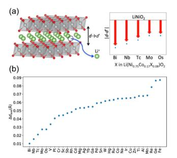
Fig. 6 (a) Representation of layer distance variation as a function of different LNO dopings. (b) Evaluation of c-axis contractions induced by 75% charging in terms of  $\Delta d_{ave}$  as a function of doping element. Lower vertical axis values indicate smaller expected contraction and improved cycle performance. Adapted from ref. 126. Copyright 2019, American Chemical Society.
