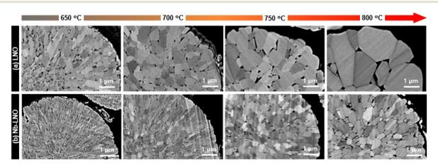
Fig. 9 Cross-sectional SEM images of (a) as-prepared LNO and (b) Nb-LNO calcined at 650-800 °C. Adapted from ref. 115. Copyright 2023, Wiley-VCH GmbH
