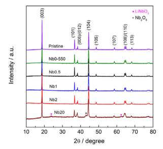
Fig. 4 XRD patterns of NCM622 coated with different loadings (wt%) of LiNbO<sub>3</sub> prepared from an ammonium niobium oxalate sol-gel method. Reproduced with permission from ref. 56. Copyright 2021, Elsevier.
