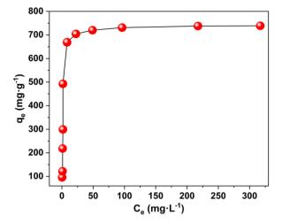
Pb<sup>2+</sup> adsorption isotherm for MOF nanosheets.
