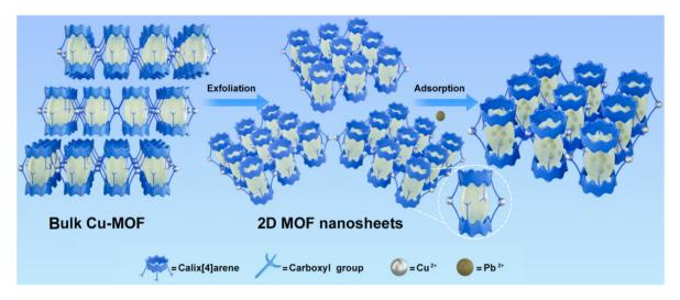
Scheme 1 Schematic illustration of the construction of 2D MOF nanosheets with cavity structures for pollutant removal.
