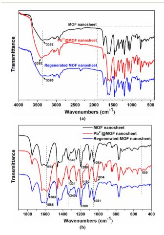
Fig. 8 Comparison of the FT-IR spectra at 400-4000 cm<sup>-1</sup> (a) and 400-1900 cm<sup>-1</sup> (b) for MOF nanosheets, Pb<sup>2+</sup>@MOF nanosheets, and regenerated MOF nanosheets.
