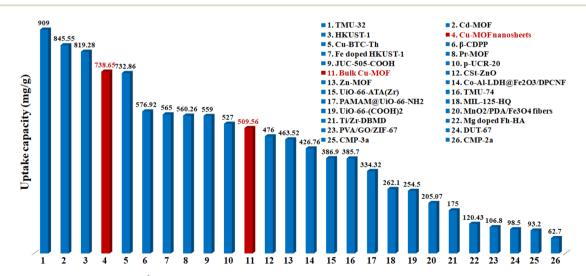
Fig. 5 Comparison of the maximum Pb2+ adsorption capacity for MOF nanosheets (no. 4) and bulk Cu-MOFs (no. 11) with various adsorbents (Table S2†).
