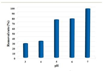
Fig. 3 pH effect on the removal efficiency of Pb<sup>2+</sup> by MOF nanosheets.  $C_0 = 10 \text{ ppm}, m_{\text{adsorbent}} = 5 \text{ mg}, V = 50 \text{ mL}, pH = 3.0-7.0.$
