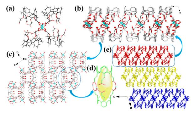
Fig. 1 (a) View of the [Cu<sub>2</sub>(HL)<sub>4</sub>(H<sub>2</sub>O)<sub>2</sub>] secondary building unit in Cu-MOFs. Color codes: cyan, Cu; red, O; gray, C; light gray, H. (b and c) View of the 2D structures in Cu-MOFs. (d) Cage-like cavity in Cu-MOFs. (e) 3D motif in Cu-MOFs.
