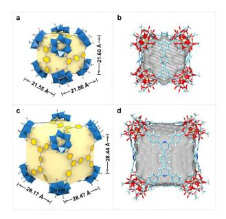
Fig. 3 Crystal structures of VMOC-4 (a and b) and VMOC-6 (c and d). The left column highlights the overall size of each cubic cage and the arrangement of the ligands, while the right column shows the void spaces (gray mesh) calculated using the VOIDOO program.
