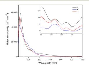
Fig. 10 UV-visible absorption spectra of heterometallic clusters 5-7 measured in THF at RT (inset: near-infrared absorption spectra).
