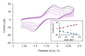
Fig. 2 Overlaid cyclic voltammograms of 1 (1 mM) in THF with 0.1 M  $N(Bu)_4PF_6$ . Scan rates = 50, 100, 200, 300, 400, 500 mV s<sup>-1</sup> referenced to a ferrocene/ferrocenium redox couple (Fc). Inset: plot of cathodic peak current ( $\bullet$ ,  $R^2 = 0.9953$ ) and anodic peak current ( $\bullet$ ,  $R^2 = 0.9962$ ) versus square root of scan rate.
