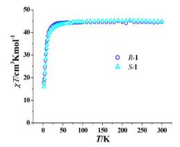
Fig. 3 Plots of  $\chi T$  versus T of R-1 and S-1 ( $H_{dc}$  = 1000 Oe).
