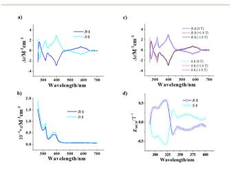
Fig. 5 CD spectra of R-1 and S-1 at room temperature (MeCN, c =0.2 g  $L^{-1}$ , optical path = 1 mm) (a). UV-visible spectra of R-1 and S-1 at room temperature (MeCN,  $c = 0.2 \text{ g L}^{-1}$ , optical path = 1 mm) (b). CD spectra in a MeCN solution at room temperature ( $c = 0.2 \text{ g L}^{-1}$ , optical path = 1 mm, H = 0 and  $\pm 1.0$  T) (c).  $g_{MCD}$  of R-1 and S-1 (d).
