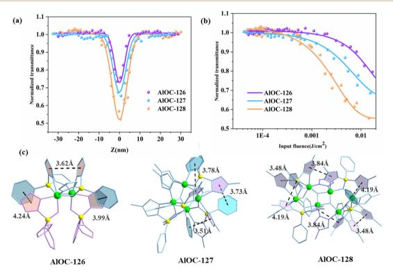
Fig. 6 (a) OA Z-scan curves and (b) OL curves of the samples at picosecond laser excitation (input energy: 4 µJ). The linear transmittance of the samples was adjusted to be 65%. Colored scattered balls indicate experimental data with the solid line representing the curve of best fit. (c)  $\pi - \pi$ interactions between adjacent L in AlOC-126, AlOC-127, and AlOC-128. Color code: Al, green; B, yellow.
