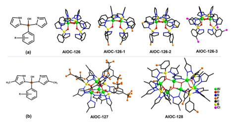
Fig. 1 A display of all compounds isolated herein showing the association of structure type and ligand regulation. (a) The alternation of functional groups on the benzene ring results in the AIOC-126 series. (b) The change on both the benzene ring and pyrazole brings the nuclearity increment, see compounds AlOC-127 and AlOC-128.
