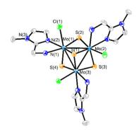
Fig. 3 ORTEP representation (50% probability ellipsoids) of the cationic cluster  $[Mo_3S_4Cl_3(ImNH_2)_3] + (1^+)$ . Hydrogen atoms have been omitted for clarity. Standard deviations of average distances are given in brackets. Average bond distances: Mo-Mo = 2.7378 [7],  $Mo-(\mu^3-S) = 2.328$  [2],  $Mo-(\mu^3)_{trans-Cl} = 2.28$  [1],  $Mo-(\mu^3)_{trans-NH_3} = 2.29$  [1] Å.
