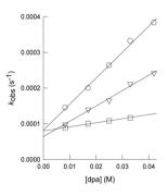
Fig. 5 Plot of the dependence with the dpa concentration of the observed rate constants for the reaction of clusters [1]BF<sub>4</sub> (circles), [2] BF<sub>4</sub> (triangles), and [3]BF<sub>4</sub> (squares), with an excess of dpa in CH<sub>3</sub>CN solutions at 25 °C.
