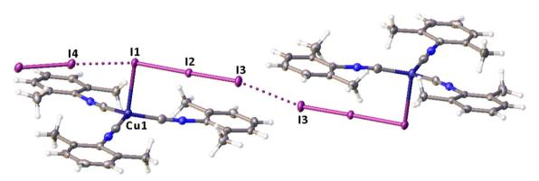
Fig. 3 Two types of I...I contacts in the structure of  $2 \cdot \frac{1}{2} I_2$ .
