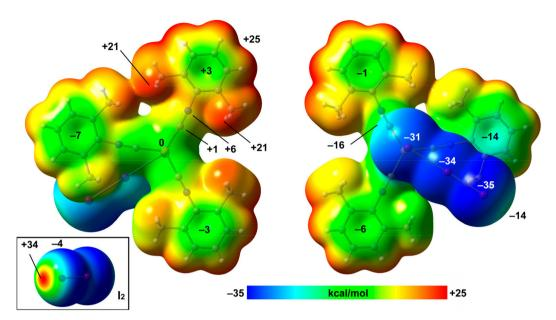
Fig. 7 MEP surfaces (two opposite orientations) of compound 2 and iodine (bottom-left). The energies at selected points of the surfaces are given in kcal mol<sup>-1</sup>. Isosurface 0.001 a.u. the PBE-D3/def2-TZVP level of theory.
