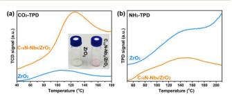
Fig. 3 (a)  $CO_2$ -TPD of  $C_{16}N-Nb_6/ZrO_2$  and  $ZrO_2$ , inset: optical photographs of C<sub>16</sub>N-Nb<sub>6</sub>/ZrO<sub>2</sub> and ZrO<sub>2</sub> slurry after adding phenolphthalein. (b) NH<sub>3</sub>-TPD of C<sub>16</sub>N-Nb<sub>6</sub>/ZrO<sub>2</sub> and ZrO<sub>2</sub>.
