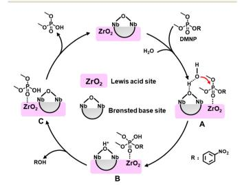
Fig. 7 The possible hydrolytic degradation mechanism for DMNP on the C<sub>16</sub>N-Nb<sub>6</sub>/ZrO<sub>2</sub> catalyst.
