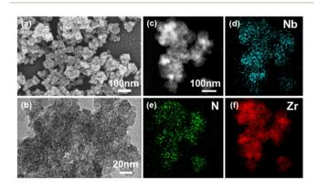
Fig. 2 (a) SEM image, (b) TEM image, (c) HAADF-STEM image, and (d-f) EDX elemental mappings of the C<sub>16</sub>N-Nb<sub>6</sub>/ZrO<sub>2</sub> composite.
