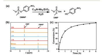
Fig. 4 (a) Catalytic hydrolysis reaction of the phosphonate-based nerve agent simulant DMNP using C<sub>16</sub>N-Nb<sub>6</sub>/ZrO<sub>2</sub>; (b) <sup>31</sup>P NMR of DMNP hydrolysis catalyzed by  $C_{16}N-Nb_6/ZrO_2$  at various intervals of time; (c) time profile for DMNP degradation. Reaction conditions: DMNP (5 mg),  $H_2O$  (300  $\mu$ L),  $CD_3CN$  (200  $\mu$ L),  $C_{16}N-Nb_6/ZrO_2$  (15 mg), and room temperature for 6 h.
