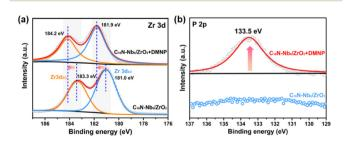
Fig. 6 High-resolution XPS spectra of the C<sub>16</sub>N-Nb<sub>6</sub>/ZrO<sub>2</sub> composite treated with DMNP in a non-aqueous system: (a) Zr 3d and (b) P 2p.
