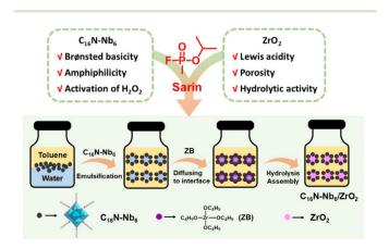
Scheme 1 Illustration of the design and fabrication of the C<sub>16</sub>N-Nb<sub>6</sub>/ ZrO<sub>2</sub> composite using an emulsion assisted self-assembly approach.
