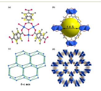
Fig. 1 The structure of Ni-MOF1. (a) The coordination environment of inorganic SBUs. (b) The cage structure. (c) The 6-connected topology network. (d) View of the 3D structures along the c axis (blue balls: Ni; red balls: O; yellow balls: S; and grey balls: C).
