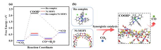
Fig. 5 The DFT results and possible mechanism. (a) Free energy profile for the CO₂RR on Ni-MOF1 and Ru complex/Ni-MOF1 (the free energy zero is set as that of a CO<sub>2</sub> molecule in the gas phase and the catalyst). (b) Synergistic effect of a CO<sub>2</sub> bridged photocatalytic interface of the Ru complex and Ni-MOF1.
