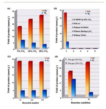
Fig. 3 CO<sub>2</sub> photoreduction performance and recycling. (a) Ni-MOF1 under different CO<sub>2</sub> concentrations. (b) Ni-MOF1 under various reaction conditions. (c) Cycling tests under 3 h of irradiation in a 10% CO2 atmosphere over Ni-MOF1. (d) The yield of CO and H<sub>2</sub> on Ni-MOF1 in real flue gas.
