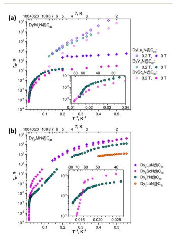
Fig. 10 Magnetization relaxation times of the  $DyM_2N@C_{80}$  series (a; M = Sc, Lu, Y; field 0 T and 0.2 T) and  $Dy_2MN@C_{80}$  series (b; M = Sc, Lu, Y, La; field 0 T). Insets show enlargement of high-temperature parts. The data for M = Sc are from ref. 72 ( $DySc_2N$ ) and ref. 71 ( $Dy_2ScN$ ), for M = Lu - from ref. 24.
