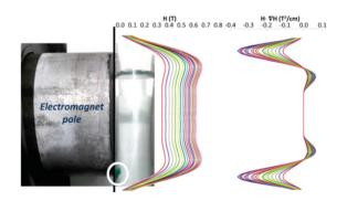
Fig. 7 Magnetic field profile [H and  $H \cdot \nabla(H)$ ] on the electromagnet pole along the dashed line. The different colours refer to the applied intensity current: increasing from 0.0 to 2.5 A (step: 0.1 A).
