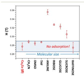
Fig. 10 Measured critical magnetic field at which the  $Cu_6Cu$  particles are detached from the pole of the electromagnet after the sorption experiment in aqueous solutions of a series of substances.  $\emptyset$  indicates control experiment using pure water.
