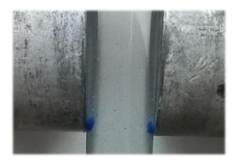
Fig. 6 Cu<sub>6</sub>Zn particles attached to the poles of the electromagnet while submerged in water.
