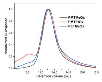
Fig. 2 SEC traces of the homopolymers eluted with DMAc/LiCl.
