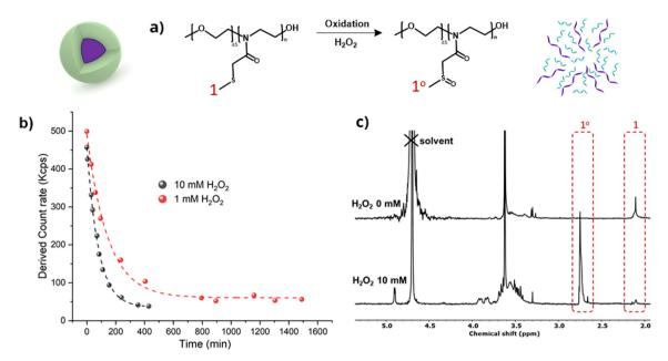
Fig. 7 (a) Schematic illustration of the oxidative reaction of PEG-b-PMTMeOx (DP = 30) block copolymer NPs with H<sub>2</sub>O<sub>2</sub>, (b) decrease of DLS scattering light intensity of the nanoparticle solution at 1 mg mL<sup>-1</sup> when adding 1 and 10 mM H<sub>2</sub>O<sub>2</sub> and (c) <sup>1</sup>H NMR spectra of PEG-b-PMTMeOx before and 24 hours after oxidation with 10 mM H<sub>2</sub>O<sub>2</sub> in D<sub>2</sub>O.
