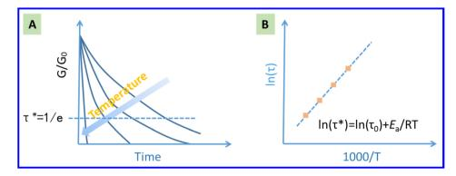
Fig. 6 A: Stress-relaxation curves commonly used to monitor the network exchange of CANs. B: Arrhenius plot of  $\ln(r^*)$  against the inverse of temperature.
