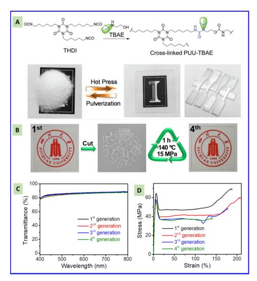
Fig. 8 Optical images showing the reprocessing process of a polyurea containing tert-butyl as a hindered group (A) and acylsemicarbazide group. Reproduced from ref. 157 with permission from John Wiley and Sons, copyright 2016. (B) Optical (C) and mechanical (D) properties of a polyacylse-micarbazide after being reprocessed four times. Reproduced from ref. 87 with permission from the American Chemical Society, copyright 2020.
