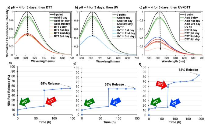
Fig. 5 Fluorescence spectra of Nile Red loaded, worm-like TORC-NGs after acidification to pH = 4 with HCl and incubating for 3 days followed by addition of DTT alone (c = 51.1 M; a, d), irradiation with 254 nm UV light for 1 h alone (b, e), or introduction of UV light and DTT sequentially (c, f) leading to AND-gate cargo release only when both stimuli were applied.
