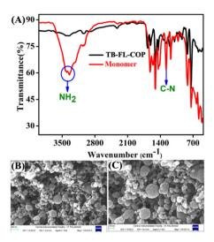
Fig. 1 (A) The FT-IR spectrum of polymer TB-FL-COP and monomer. The FESEM images of TB-FL-COP were imaged at (B) 100 and (C) 200 nm resolutions.
