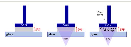
Fig. 15 Schematic representation of the shrinkage measurement apparatus.
