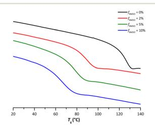
Fig. 6 Thermograms from DSC analyses performed on the dried extract of latexes of PMMA (E1MMA) and P(MMA-co-BMDO) with increasing amounts of BMDO:  $f_{\rm BMDO,0}=2\%$  (E4BMDO),  $f_{\rm BMDO,0}=5\%$  (E1BMDO),  $f_{\rm BMDO,0}=10\%$  (E5BMDO) (Table 1).
