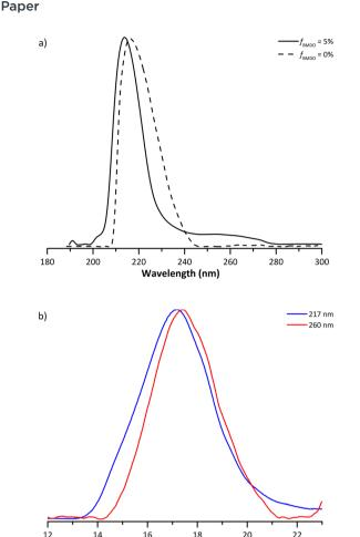
Fig. 3 (a) SEC traces from the UV detector obtained for the dried extract from experiments E1MMA ( $f_{\rm BMDO,0}$  = 0%) and E1BMDO ( $f_{\rm BMDO,0}$ = 5%, Table 1), normalized on the maximum of absorption. (b) SEC traces from the UV detector set at 217 nm (blue) and 260 nm (red) obtained for experiment E1BMDO (Table 1).
