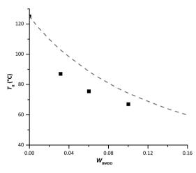
Fig. 7 Evolution of experimental (square) and theoretical (dashed line)  $T_{\rm g}$  with the mass fraction of BMDO. Theoretical values were calculated with the Fox equation.
