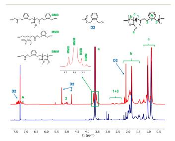
Fig. 2 <sup>1</sup>H NMR spectra of the dried extract of latexes E1BMDO (red) and E1MMA (blue) (CDCl<sub>3</sub>, 256 scans). Assignments were made according to a previous report. <sup>13</sup> B stands for BMDO units and M for MMA units in a triad. D2 corresponds to one of the identified degradation products of BMDO (see ESI, Fig. S1†).
