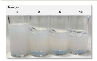
Fig. 4 Photos of the latexes prepared with different initial molar fraction of BMDO. From left to right: experiments E1MMA,  $f_{BMDO,0} = 0\%$ ; E4BMDO,  $f_{BMDO,0} = 2\%$ ; E1BMDO,  $f_{BMDO,0} = 5\%$ ; E5BMDO,  $f_{BMDO,0} = 10\%$ (Table 1).
