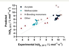
Fig. 2 The predicted *versus* experimental values of the  $\ln(k_{\rm p})$  at 25 °C for a dataset n=41 using the leave one out cross validation on a linear regression. Predictions are determined using Mr, inductive effects, DP, BPK, MPK, and GFE ( $r^2=0.631$ , RME = 1.167).
