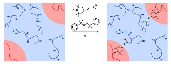
Fig. 6 TEMPO-epoxy as a proposed compatibilizing agent to stabilize the interface between PE (in red) and EVOH (in blue) phases through the grafting of the TEMPO group of TEMPO-epoxy onto PE and the coupling reaction of the epoxy group of TEMPO-epoxy with the hydroxyl groups of EVOH.
