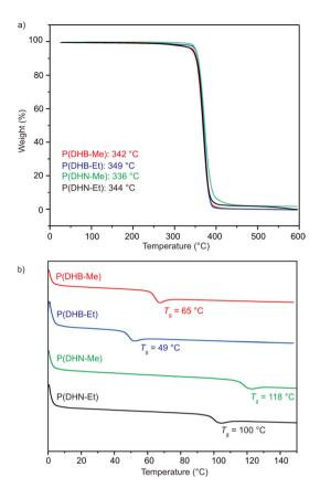
**Fig. 2** Thermal properties of the produced semiaromatic polyesters. (a) TGA curves of P(DHB-Me), P(DHB-Et), P(DHN-Me), and P(DHN-Et). (b) DSC curves of P(DHB-Me), P(DHB-Et), P(DHN-Me), and P(DHN-Et).
