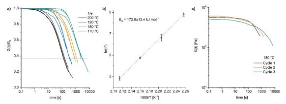
Fig. 6 (a) Normalized stress-relaxation curves obtained from **poly4** at temperatures ranging from 170 to 200 °C with 1/e (dotted line) used for the determination of the characteristic relaxation time ( $\tau^*$ ); (b) fitting of the relaxation times ( $\tau^*$ ) vs. temperature data by the Arrhenius equation for **poly4**; (c) non-normalised stress-relaxation curves obtained from **poly4** measured repeatedly at a temperature of 180 °C.
