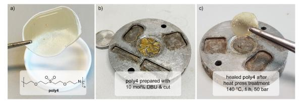
Fig. 5 (a) Membrane of poly4 prepared from 1 equiv. divinyl sulfone, 0.66 equiv. triethanolamine and 0.10 equiv. DBU; (b) photograph of a cut membrane of poly4 placed in mould; (c) photograph of a membrane of poly4 obtained from cut pieces shown in b after hot press treatment (140 °C, 1 h, 50 bar).
