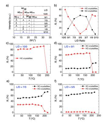
Fig. 4 (a) PXRD patterns of HC- and SC-PLA microspheres. (b) The relative degree of crystallinity  $(X_c)$  of the HC and SC crystallites. (c-f)Relative degree of  $X_c$  versus temperature in the range of 25 to 220 °C for HC and SC crystallites of PLA with L/D ratios of 10/0 (c), 9/1 (d), 7/3 (e), and 5/5 (f).
