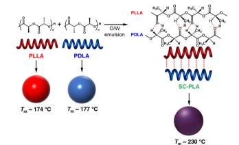
**Fig. 1** Schematic illustration of the fabrication of microspheres from HC- and SC-PLA by the O/W miniemulsion method.
