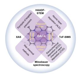
Fig. 2 Illustration of the preparation and characterization methods of DACs. HAADF-STEM: high-angle annular dark-field scanning transmission electron microscopy; XAS: X-ray absorption spectroscopy; ToF-SIMS: time-of-flight secondary ion mass spectrometry.
