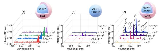
Fig. 2 Anti-Stokes emission spectra of β-NaYF<sub>4</sub> nanocrystals: (a) core-shells singly doped with  $Pr^{3+}$  ions; (b) cores co-doped with  $x\%Pr^{3+}$ ,  $15\%Yb^{3+}$ ; (c)  $x\%Pr^{3+}$ ,  $15\%Yb^{3+}$  co-doped cores with a passive shell with assigned transitions. The presented emission spectra were recorded under 852 nm excitation (1.5 MW cm<sup>-2</sup>) at room temperature.
