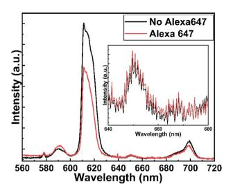
Fig. 6 Emission spectra from two different areas on Eu-HQA + Alexa647 surface: pristine Eu-HQA area without Alexa647 and area within which an Alexa647 droplet is located.
