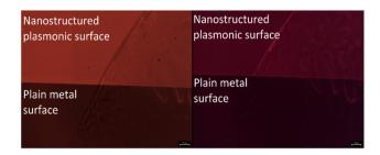
**Fig. 5** Fluorescence microscope images: (left) 615 nm Eu<sup>3+</sup> emission, and (right) 660 nm FRET emission, obtained for Eu-HQA + Alexa647 surfaces on nanostructured plasmonic surface (top) and on plain metal surface (bottom). The tilted lines in the images represent the left-side edge of the Alexa647 droplet.
