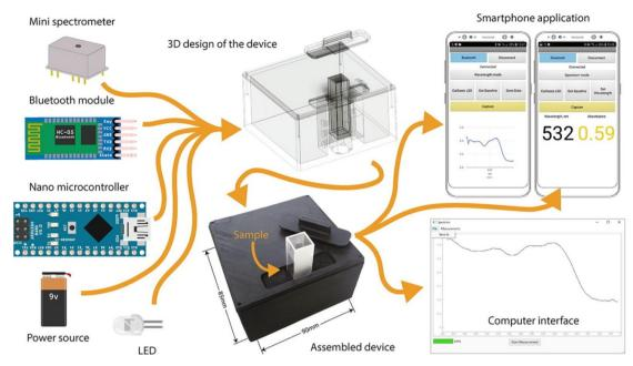
Fig. 8 Portable handheld colorimetric detection of phosphate [this figure has been reproduced from ref. 37 under open access article in terms of the Creative Commons CC-BY licensel
