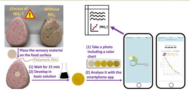
Fig. 12 Smartphone-based colorimetric determination of the nitrite ion in a meat sample [reprinted from ref. 40 with permission from American Chemical Society].
