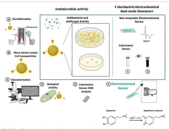
Fig. 7 CuO-Maca NP-based portable colorimetric/electrochemical sensing of dopamine using the paper-based smartphone sensing technique. (A) Synthesis of CuO-Maca by a sonication method. (B) Image of Maca-CuO NPs. (C) Characterization of CuO-Maca. (D) Antibacterial activity check using CuO-Maca. (E) Smartphone-assisted colorimetric sensing. (F) Portable electrochemical sensing of dopamine [this figure has been reproduced from ref. 70 with permission from Elsevier Sciences, copyright 2022].
