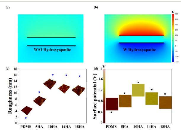
Fig. 3 (a and b) Comsol simulations with and without hydroxyapatite. (c) Surface morphology and (d) surface potential of HA/PDMS bionanocomposite films were obtained by AFM.
