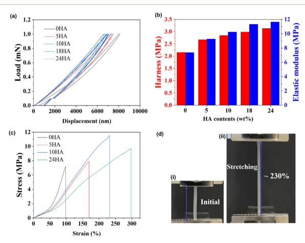
Fig. 2 (a) Load-displacement (depth) curve of HA/PDMS thin film via nanoindentation. (b) Harness and elastic modulus of HA/PDMS with different contents of hydroxyapatite. (c) Tensile stress-strain curve of HA/PDMS bionanocomposite with different hydroxyapatite contents. (d) Digital image of 10HA/PDMS before and after stretching.
