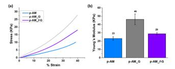
Fig. 6 (a) Stress-strain curves and (b) Young's modulus of p-AM hydrogels.
