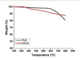
Fig. 1 TGA analysis of FLG vs. f-FLG.
