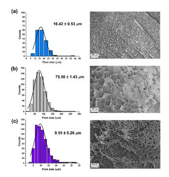
Fig. 5 Pore-size distribution and SEM images of (a) blank, (b) FLG and (c) f-FLG p-AM hydrogels.
