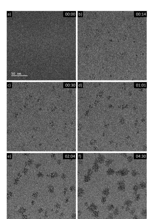
Fig. 1 Sequential images from an *in situ* LP-TEM movie showing the formation of aggregates (see video "V01\_LP-TEM\_CeO<sub>2</sub>-nanoparticles.avi", time given as mm:ss). A dose rate of  $16.7 \times 10^6$  Gy s<sup>-1</sup> is applied.
