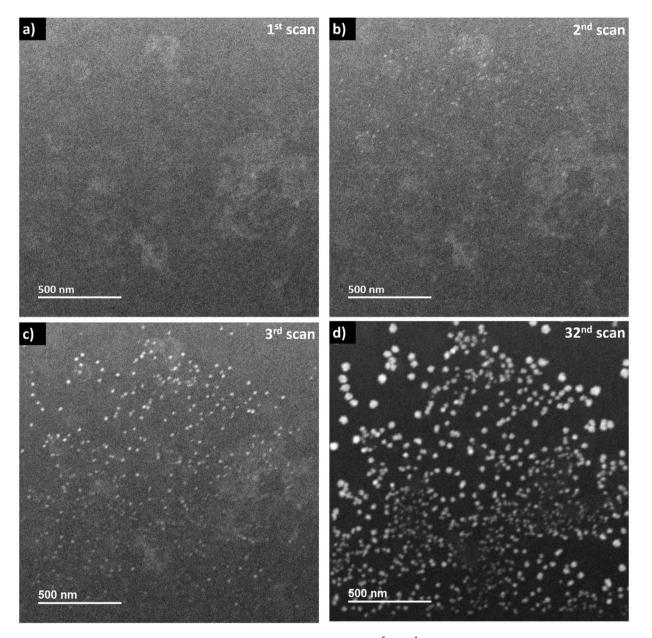
Fig. 6 Sequential *in situ* ADF imaging in LP-STEM. An averaged dose rate of  $2.4 \times 10^5$  Gy s<sup>-1</sup> is applied. (a) Initial scan. (b) Nano-sized aggregates become visible in the second scan and (c) their contrast increases during exposure. (d) The projected size of the aggregates increases constantly while almost no new ones are formed. (see video "V04\_LP-STEM\_CeO<sub>2</sub>-nanoparticles.avi").
