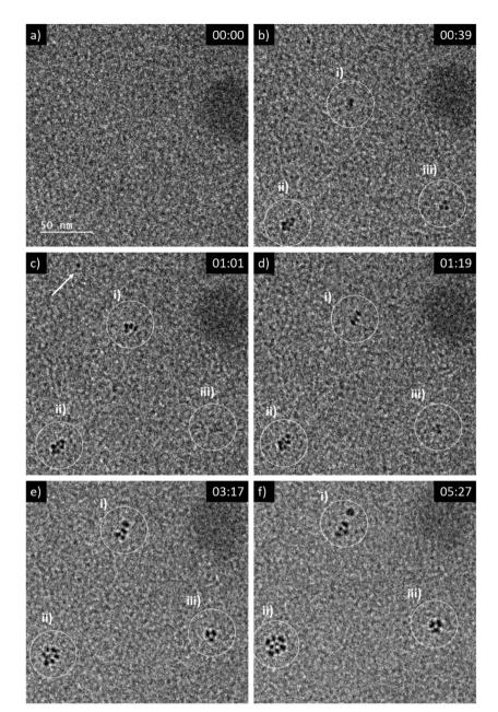
Fig. 2 Sequential images from an *in situ* LP-TEM movie showing (a)–(b) formation and (c)–(f) arrangement of primary particles when a dose rate of  $16.7 \times 10^6$  Gy s<sup>-1</sup> is applied. Primary CeO<sub>2</sub> particles can be resolved and evaluated quantitatively, because of lower thickness of the liquid in comparison to Fig. 1. (See also according video "VO2\_LP-TEM\_CeO<sub>2</sub>-nanoparticles"; time given as mm:ss).
