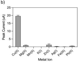
Fig. 4 DPV response curves of polydopamine entrapped F8-DNAzyme electrode, polydopamine entrapped W8-DNA (non-enzymatic) electrode and polydopamine only electrode (a) in PBS with 10 µM Cu(II) after 15 min. (b) Peak current of DPV response curves for polydopamine entrapped F8-DNAzyme electrochemical sensor in 1 times PBS with 10 μM of Cu(ii), Mg(ii), Mn(ii), K(i), and Zn(ii), Ag(i), Fe(iii), and Pb(ii) after 15 min.
