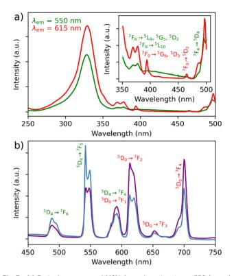
Fig. 3 (a) Excitation spectra of MSN-1 monitored at  $\lambda_{em}=550$  (green) and  $\lambda_{em}=615$  nm (red) recorded in the solid state at RT. Inset: magnification of the excitation spectra between 340 and 510 nm. (b) Emission spectra of MSN-1 recorded at 77 K (blue) and room temperature (violet) in the solid state with excitation at  $\lambda_{em}=328$  nm. Eu<sup>3+</sup> and Tb<sup>3+</sup>-linked transitions are shown in red and green, respectively.
