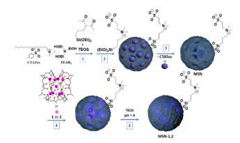
Scheme 1 Schematic representation of the synthesis of functionalized hybrid nanoparticles MSN-1 and MSN-2. The used complexes 1 or 2 are  $[(Tb/Eu)_9(acac)_{16}(\mu_3-OH)_8(\mu_4-O)(\mu_4-OH)]\cdot H_2O$  (where Tb/Eu ratio = 19/1 for 1 and 9/1 for 2).
