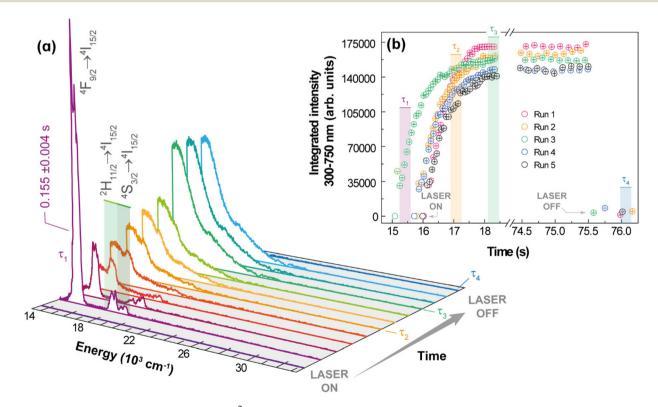
Fig. 6 Emission spectra of 1 acquired at 102 W·cm<sup>-2</sup> under ambient conditions. (b) Transient integrated intensity over 300 at 750 nm (see text for the meaning of  $\tau_1$ ,  $\tau_2$ ,  $\tau_3$ , and  $\tau_4$ ).
