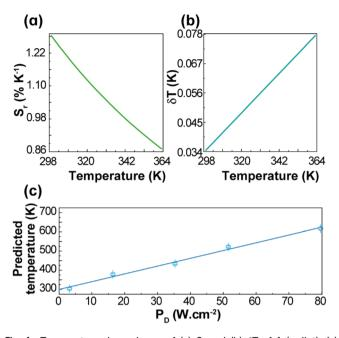
Fig. 4 Temperature dependence of (a)  $S_r$  and (b)  $\delta T$  of 1 (pellet). (c) Dependence of the predicted temperatures on  $P_D$  for 1 (pellet). The line is the best linear fit to the data ( $r^2 > 0.985$ ).
