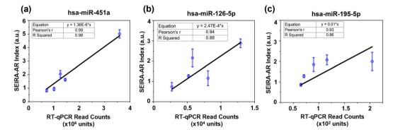
Fig. 7 SEIRA-AR index values correlation with RT-qPCR data for (a) hsa-miR-451a, (b) hsa-miR-126-5p, and (c) hsa-miR-195-5p. The data points in blue show the mean and standard deviation values. The linear curve fitting is represented in black. The fitting equation, Pearson's *r*, and *R* Squared values are indicated in the top left corner.
