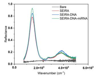
Fig. 5 SEIRA enhancement. Reflectance measurements of a bare area without SEIRA, shown as black, an area with SEIRA structures when it was clean (red), after DNA binding (blue), and after miRNA binding (green).
