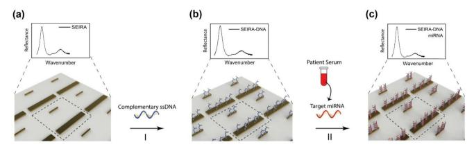
Fig. 2 Experimental workflow. (a) Measurement was performed on a clean SEIRA sensor (zoom-in view). Dashed square is a design unit cell of the SEIRA structure. (b) Step I: Complementary ssDNA (with thiol group modification) solution was immobilized onto the SEIRA substrate. Measurement was performed on the SEIRA-DNA substrate. (c) The total RNA solution containing target miRNA molecules was immobilized onto the SEIRA-DNA substrate. Measurement was performed on the SEIRA-DNA-miRNA substrate.
