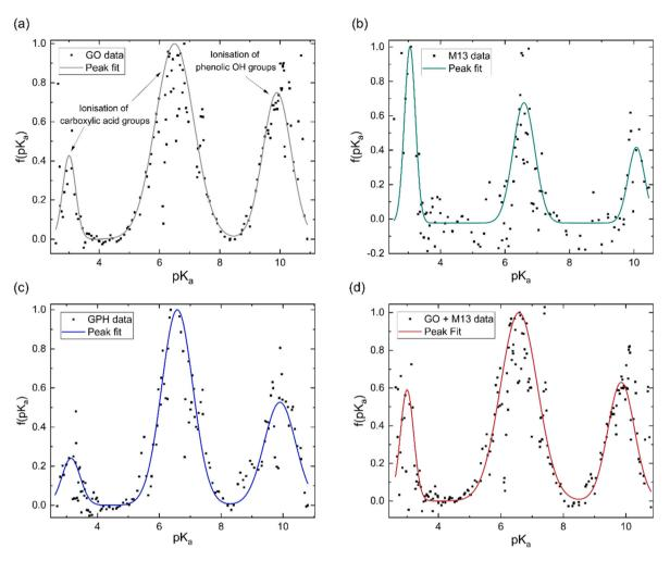
Fig. 3 Normalised  $pK_a$  distribution of (a) GO, (b) M13 bacteriophage, (c) GPH and (d) GO + M13. The peaks in (a-d) at  $pK_a$  values of 3.1 and 6.6 are due to the ionisation of carboxylic acid groups and the peak at 9.9 is due to the ionisation of phenolic OH groups (a).
