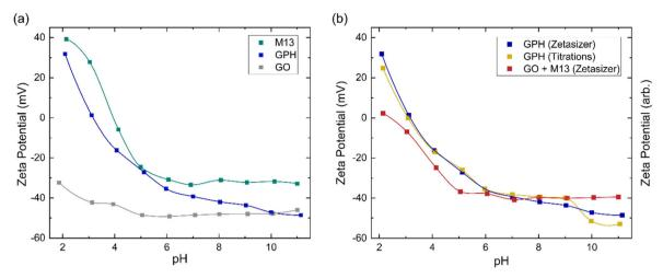
Fig. 4 (a) Zeta potential of GO, M13 bacteriophage and GPH. (b) Comparison of zeta potential measurements of GPH to the addition of the individual GO and M13 (GO + M13) along with the zeta potential trend of GPH. The trend lines are generated *via* interpolation.
