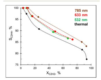
Fig. 3 Steady-state ethylene selectivity as a function of acetylene conversion over 3%Pd-Mg/GS under thermal and photo-mediated activation. The catalyst surface temperature was maintained at 60 °C for both thermal and photocatalytic experiments and the H2: C2H2 was
